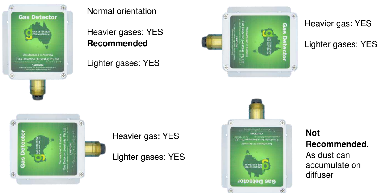
Figure 3: Sensor mounting orientation.
