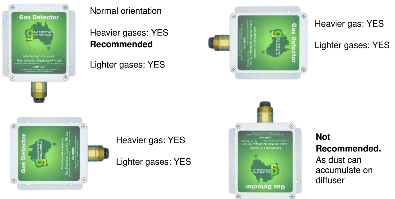
Figure 3: Sensor mounting orientation.
